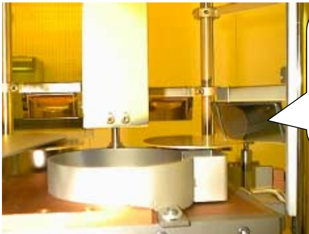
Figure 9: Side View of the Sources. Notice the shields and view mirrors.
