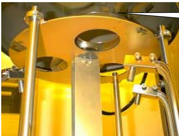
Figure 10: Target Turret. There are 3 openings for each source, one crystal monitor for each source and 2 targets.
