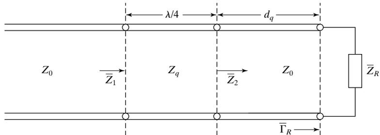
FIGURE 7.16 For illustrating the quarter-wave transformer matching technique.
