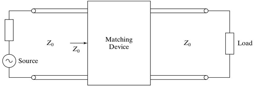
FIGURE 7.15 For illustrating the principle behind transmission-line *matching*.
