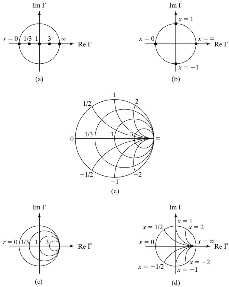
FIGURE 7.21 Development of the Smith chart by transformation from  $\bar{z}$  to  $\bar{\Gamma}$ .
