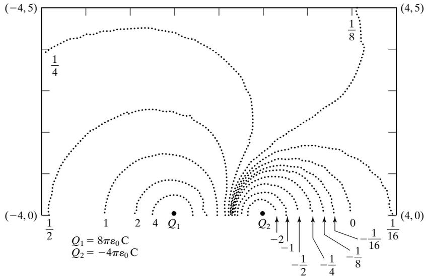
FIGURE 5.6 Personal computer-generated plot of equipotentials for the arrangement of two point charges of Fig. 5.5. The values of potentials are in volts.
