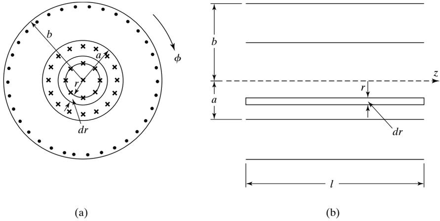
FIGURE 5.16 For evaluating the internal inductance per unit length associated with a volume current of uniform density along an infinitely long cylindrical conductor.
