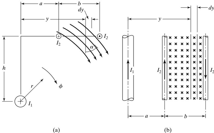
**FIGURE 5.17** For the computation of mutual inductance per unit length between a two-wire telephone line and a single wire parallel to it.
