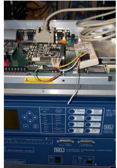
Equipment donated to the new Lab includes this data aggregator, distance relay, and test system from Schweitzer.
