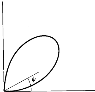
Figure 10.21. Radiation pattern in the cross-sectional plane for the case of d_1 = d_2 = \lambda/4 in the arrangement of Fig. 10.20.
