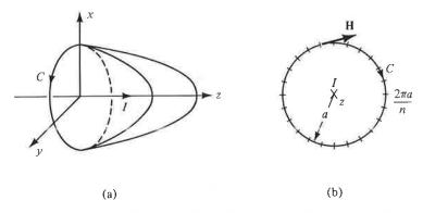
Figure 2.14. (a) For illustrating the uniqueness of a wire current enclosed by a closed path for an infinitely long, straight wire. (b) For finding the magnetic field due to the wire.
