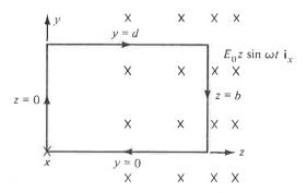
Figure 2.17. A rectangular loop in a time-varying electric field.
