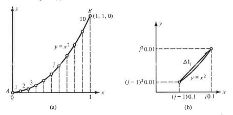
Figure 2.2. (a) Division of the path  $y = x^2$  from A(0, 0, 0) to B(1, 1, 0) into ten segments. (b) The length vector corresponding to the *j*th segment of part (a) approximated as a straight line.
