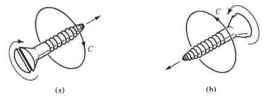
Figure 2.10. Right-hand screw rule convention employed in the formulation of electromagnetic field laws.
