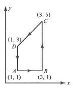
Figure 2.4. For evaluating the line integral of a vector field around a closed path.
