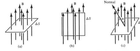
Figure 2.5. An infinitesimal surface  $\Delta S$  in a magnetic field **B** oriented (a) normal to the field, (b) parallel to the field, and (c) with its normal making an angle  $\alpha$  to the field.
