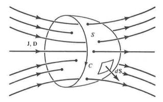
Figure 2.21. For illustrating Ampere's circuital law.
