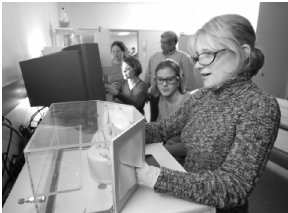
Students from the senior polymer lab characterize their samples using a Differential Scanning Calorimeter (Model: Perkin-Elmer DSC 7, foreground) and Dynamic Mechanical Analyzer (Model: Perkin-Elmer DMA 7, background).
