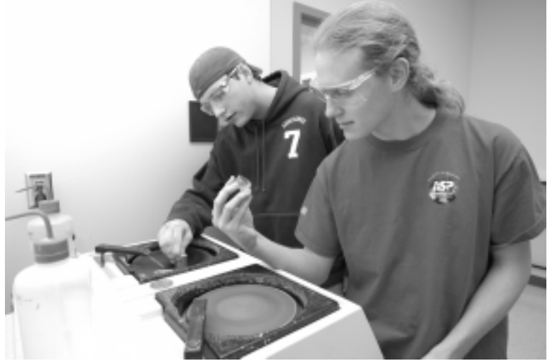
Students from the senior metals lab polish samples for micro-structural examination using a dual wheel two speed Polisher (Model: Buehler Ecomet 5)
