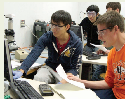
Teng-Sing Wei and Tom Quinn observe what happens when a binary organic alloy is heated and cooled. They view the image on the computer which is live fed from a CCD camera attached to an optical microscope.
