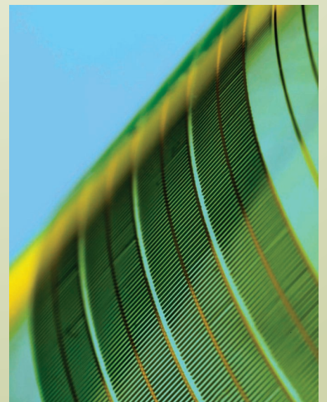
Mechanically flexible solar module formed with interconnected arrays of monocrystalline silicon microcells. This class of technology could expand the use of silicon in photovoltaics.
