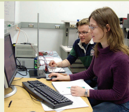
Lars Bjaalie and Suzanne Sullivan measure the difference in temperature created by running different currents through a thermoelectric material in the junior lab.
