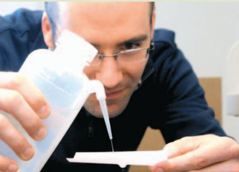
Jim Langer of Serionix pours water through filter material designed to remove the rocket-fuel component perchlorate. A grant will help the firm commercialize the technology for removing perchlorate and other contaminants.
