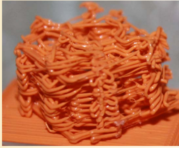
Bio-scaffolding developed for a senior design project. This is used to allow cells to migrate into the structure and study how different chemical, physical and biological cues and influence cellular identity. Photo by Jacqueline Handley.
