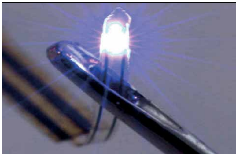
A thin plastic ribbon printed with advanced electronics is threaded through the eye of an ordinary sewing needle.
