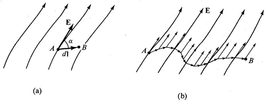
Fig. 2.21. Movement of a test charge in an electric field.
