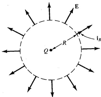
Fig. 2.4. The electric field of a point charge.
