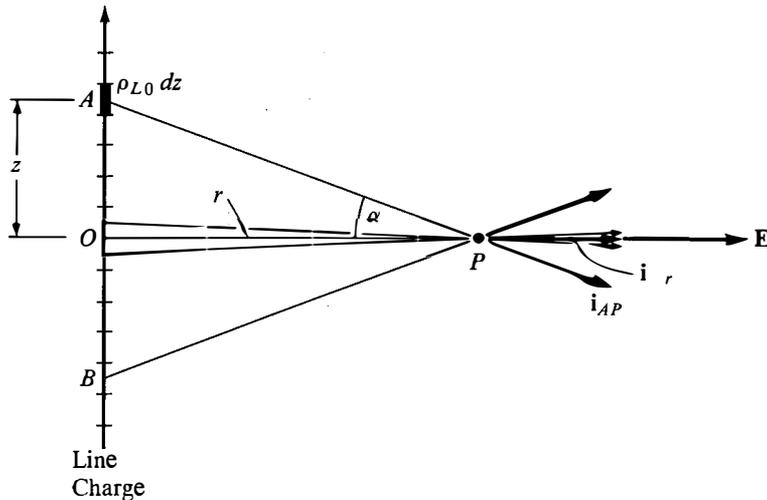
**Fig. 2.8.** Geometry for computing the electric field of an infinitely long line charge of uniform density  $\rho_{L0}$  C/m.
