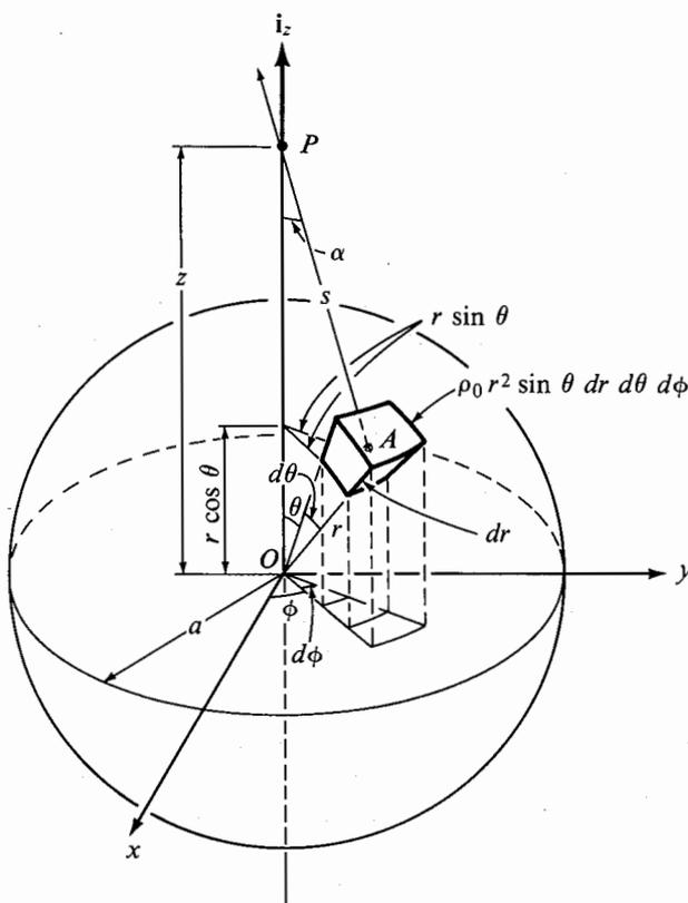
**Fig. 2.10.** Geometry for computing the electric field of a spherical volume charge of uniform density  $\rho_0$  C/m<sup>3</sup>.
