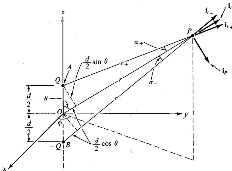
**Fig. 2.7.** Geometry pertinent to the computation of the electric field due to a dipole.
