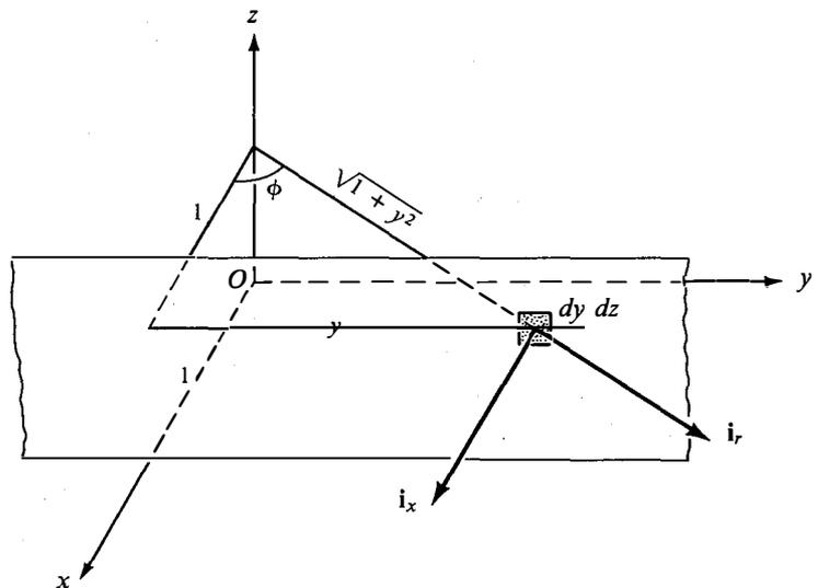
**Fig. 2.16.** For evaluation of electric field flux emanating from an infinite line charge and cutting a portion of the  $x = 1$  plane.
