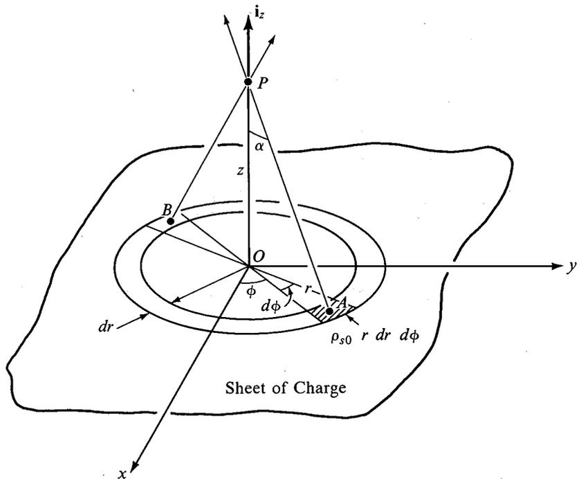
**Fig. 2.9.** Geometry for computing the electric field of an infinite sheet charge of uniform density  $\rho_{s0}$  C/m<sup>2</sup>.
