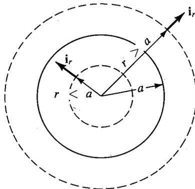
Fig. 2.19. Gaussian surfaces for computing the electric field of a spherical volume charge of uniform density.
