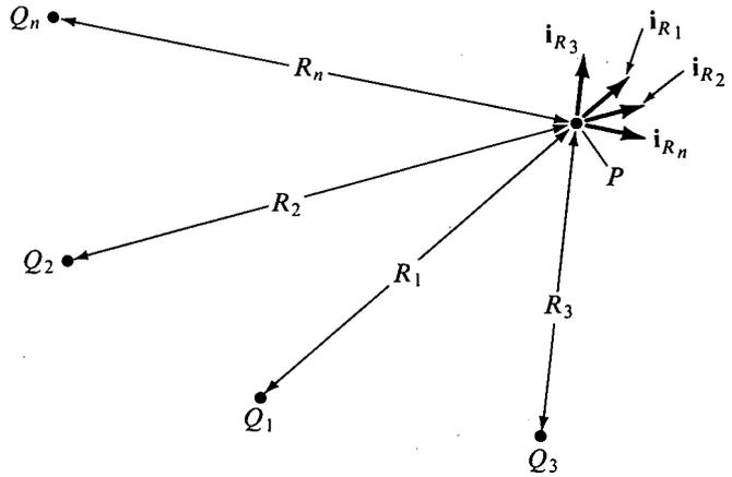
Fig. 2.5. Assembly of point charges and unit vectors along the direction of their electric field intensities at point  $P$ , due to the individual point charges.
