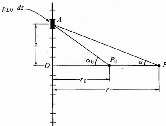
Fig. 2.27. Geometry for the computation of the potential field of an infinitely long line charge of uniform density  $\rho_{L0}$  C/m.
