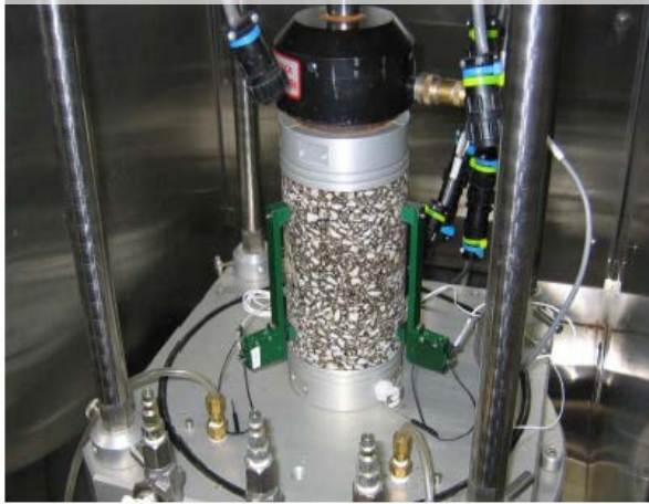
Complex Modulus Test
