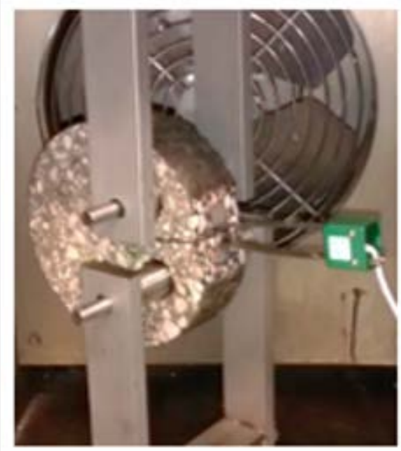
Disk Shaped Compact Tension (DCT)
