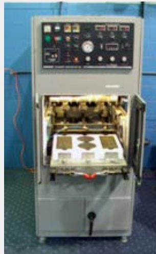
Asphalt Pavement Analyzer (APA)
