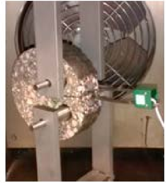
Disk Shaped Compact Tension (DCT)
