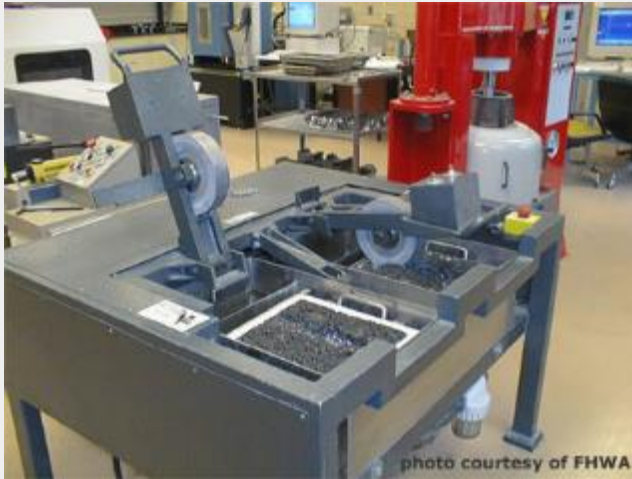
Lab Test (Hamburg Wheel Tracker)
