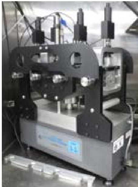
Bending Beam Fatigue
