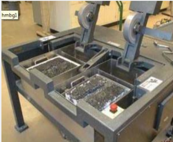
Hamburg Wheel Test (HWT)
