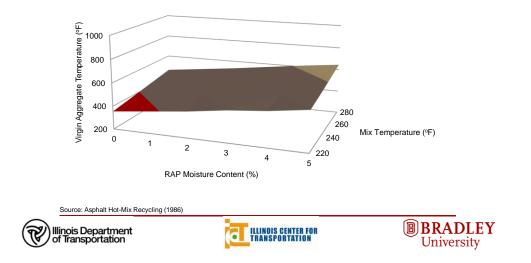
**Batch Plant: Virgin Aggregate Temperature**
