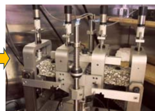
Test Specimen (380 x 63 x 50) mm
