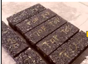
Compacted Sample (380 x 125 x 75) mm
