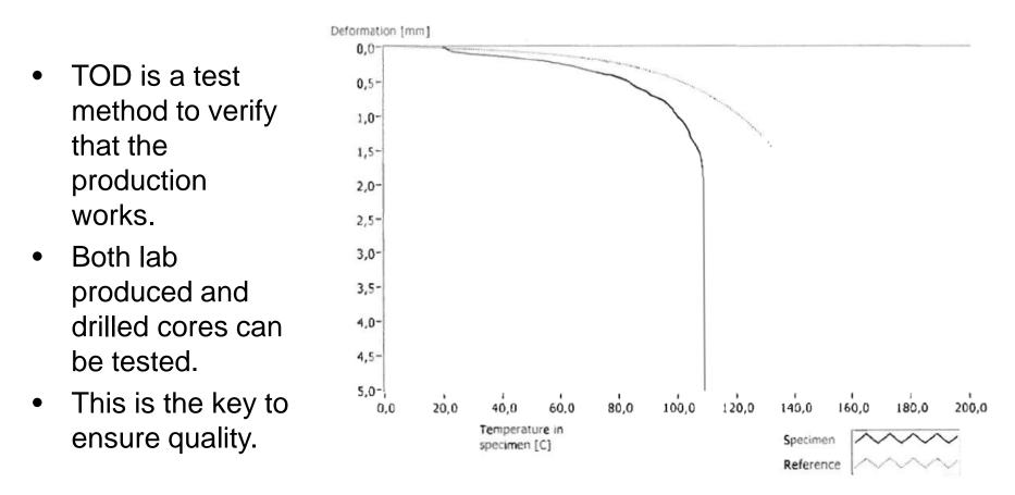
The TOD test provide a measure of viscous deformation in the specimens.
