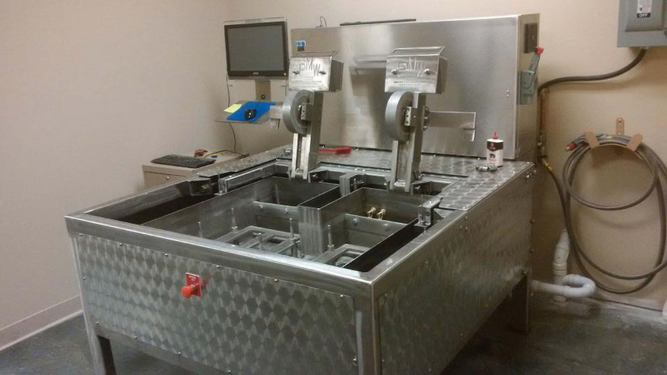
**Contractor Designs** Hamburg **Rutting Potential** SCB (Semi-Circular Bend) Cracking (Brittleness Test)
