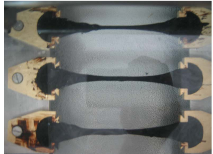
Ductility test of lumpy Pmb!
