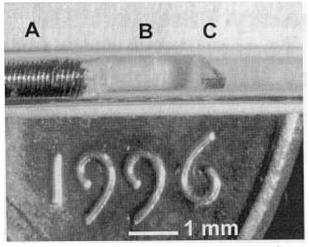
FIGURE 1. A photograph of the OCT catheter. The OCT catheter, shown with a penny and scale bar for comparison, is 1 mm in diameter. The catheter sheath remains stationary while a cable (A) rotates an optical fiber that transmits the OCT signal. A rectangular prism (B) focuses the light, and the triangular mirror (C) reflects the light radially.
