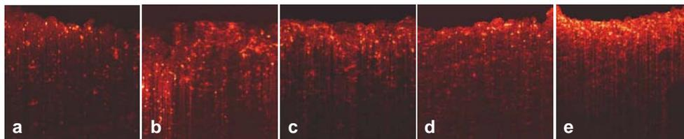
Fig. 8. Collagen-dependent changes in OCT. OCT images of tissue models are shown with a constant cell number ( $\sim 5 \times 10^4$ ) and increasing amounts of collagen in the Matrigel matrix. Collagen percentage varies for (a) 0%, (b) 0.05%, (c) 0.1%, (d) 0.15%, and (e) 0.2%. Increasing collagen content increases scattering, reducing imaging depth and contrast between cells and matrix. Scale bar represents 100  $\mu\text{m}$ .
