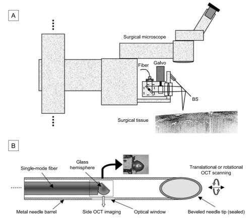
*Figure 2.* Beam-delivery systems for OCT. The OCT imaging beam can be passed through a number of existing or modified optical instruments including (A) surgical or research microscopes, and (B) fine-needle aspiration and core-needle biopsy probes, among others. Abbreviations: BS, dichroic beamsplitter; Galvo, galvanometer scanner.
