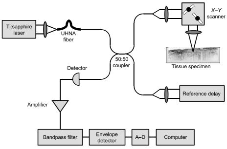
*Figure 1.* OCT schematic. The OCT technology can be fiber-optic-based, enabling a compact and portable system for use in research, clinical, and surgical settings. Abbreviations: A–D, analog-to-digital converter; UHNA, ultra-high-numerical aperture.
