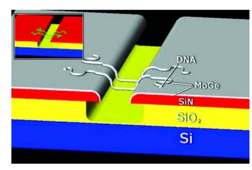
Figure 1. Diagram of a sample wafer with suspended DNA "bridges." The inset shows the strands of DNA suspended over an undercut trench in the substrate before sputtering. The sample is coated with MoGe, a superconducting metal, to make two nanowires.
