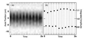
Fig. 2. M-mode OCT imaging. (a) Repetitive axial scans at 10 Hz of a magnetite microparticle embedded within 5% agarose gel during magnetic-field modulation. Each axial scan was acquired with the magnetic field alternately on and off. (b) Integrated demodulated OCT signal amplitude for each axial scan in (a). Magnetically induced displacement of the magnetic particle and subsequent restoration by the agarose medium account for the observed regularity in the modulation of the optical scattering.
