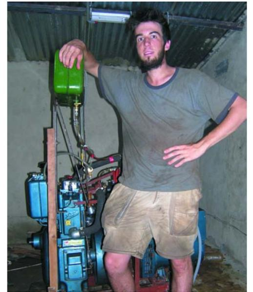
Walsh with the completed generator; his right arm is resting on the vegetable oil tank. Note the two fuel tanks—the engine starts on conventional diesel fuel to warm up the cylinder for one minute, and then a valve switches over to the vegetable oil fuel.
