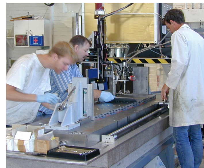
A physics undergrad works with Professor Steven Errede (right) and technician Dave Forshier (middle) to produce a TileCal submodule for the ATLAS project in 1999. A large team of undergraduates worked on the project, to produce a total of 193 TileCal submodules. This represents just one phase of the Illinois team’s contributions to the project.
