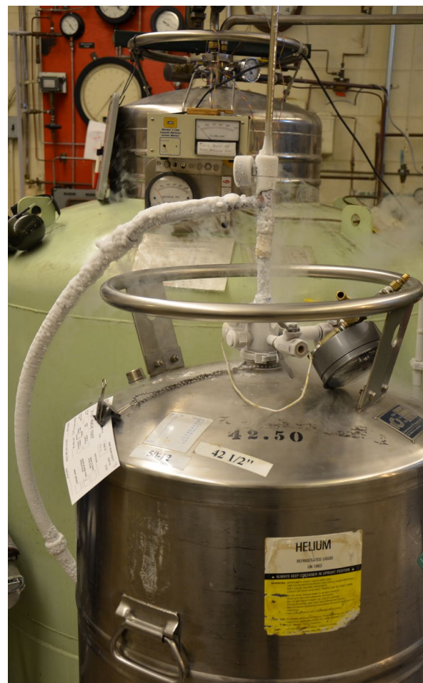
Liquid helium is collected in a 1,000-l storage dewar following liquefaction of helium gas in the department’s Linde 1410 Helium Liquefier. It takes 26.63 cu. ft. of gas to make 1 l of liquid helium.
