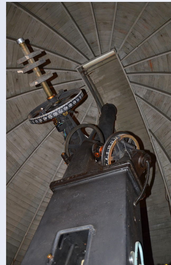
Above: The observatory's original 12-inch Brashear refractor telescope prior to disassembly and removal Below: The exterior of the 117-year-old observatory today looks much the same as when it was first erected, but for some telltale signs of age.
