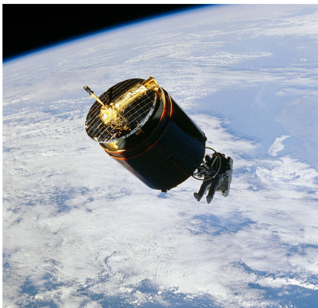
Astronaut Dale A. Gardner, getting his turn in the Manned Maneuvering Unit, prepares to dock with the spinning WESTAR VI satellite during the STS-51A mission in 1984. Gardner used a large tool called the Apogee Kick Motor Capture Device to enter the nozzle of a spent WESTAR VI engine and stabilize the communications spacecraft sufficiently to capture it for return to Earth in the cargo bay of the space shuttle Discovery. Image courtesy of NASA
