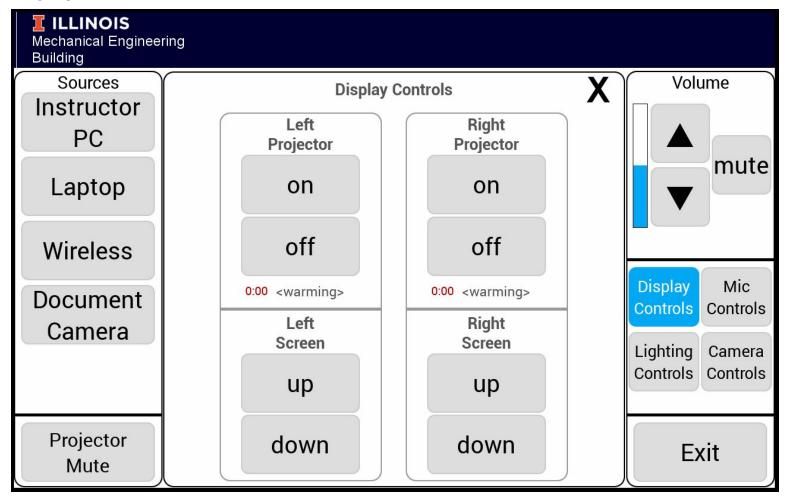
The additional selection for display controls is a convenience in the event that a projector does not automatically turn on with a source selection.
