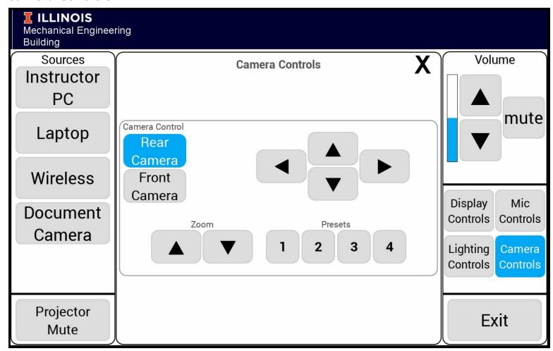
The "Lecture Capture" system uses the Extron SMP 352 and allows the user to configure the video being recorded during a classroom session. The user should consider simultaneous "Content" and "Camera" source selections that will be composited into a single layout for recording.
