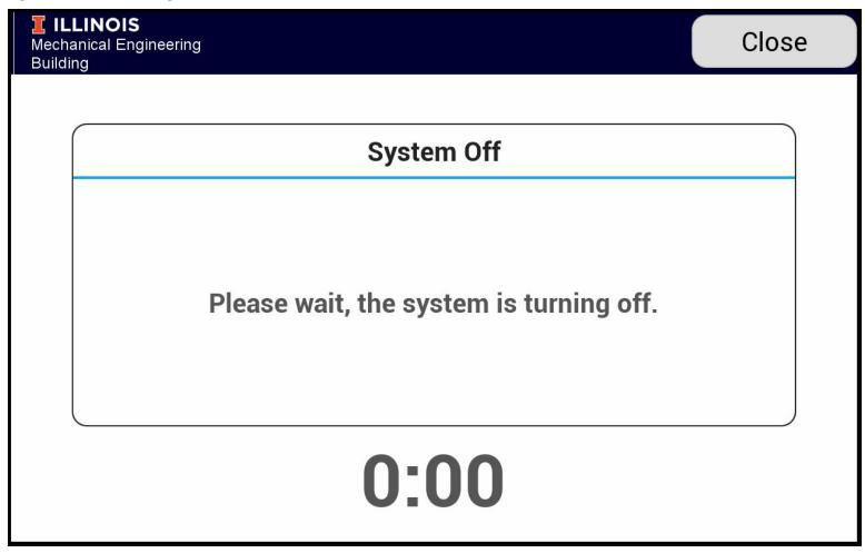
When the system is turned off, the user is prompted to wait while the equipment is turning off. This delay will generally be the time it takes for the displays to turn off and cool down.
