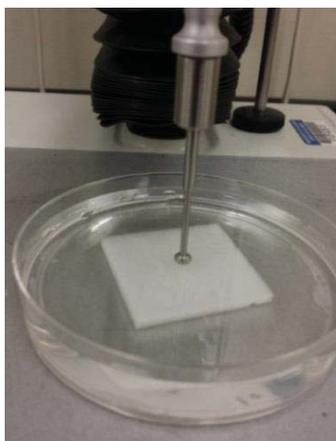
Figure 4.2: 20x20x5 mm collagen scaffold placed in petri dish over 3 grams of PDMS and submerged with PBS.
