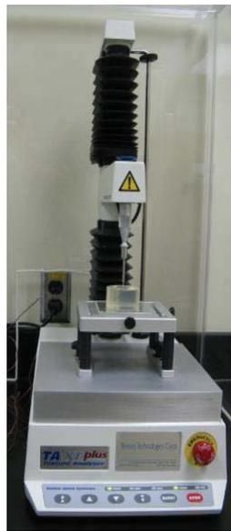
Figure 3.2: TA.XT plus Texture Analyzer used for all indentation experiments.
