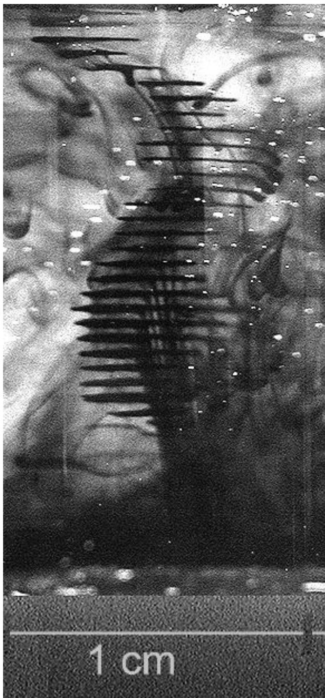
**Figure 32.** Column formation of food coloring dye using transducer II. Drive voltage was at 22.5 volts peak-peak.
