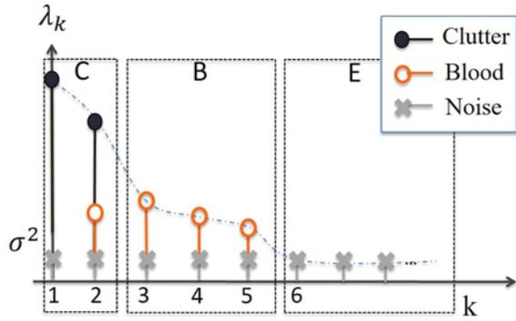
Fig. 5. A simplified eigen-spectrum of Doppler echo-signal vector  $\mathbf{x}_m$  where eigenvalues  $\lambda_k$  are sorted in decreasing order. Values are grouped into sets,  $C$ ,  $B$  and  $E$ , that approximate the three sources contributing to  $\Sigma_x$ .
