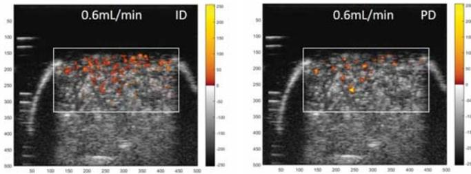
Fig. 10. Conventional power-Doppler image of phantom perfusion at 0.6 ml/min (right) and that obtained using the ID estimator (left) for the same recorded echo data. Results are coded in color and overlaid on the B-mode image. The image is a cross sectional view of the dialyzer cartridge diagrammed in Fig. 1.
