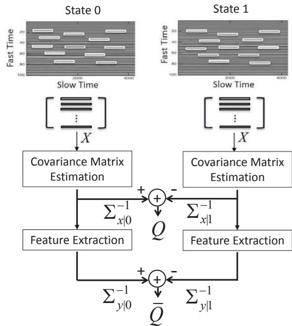
Fig. 2. Illustration of the procedure for generating data matrices  $\mathbf{X}$  and covariance matrices  $\Sigma_{x|i}$ . From covariance matrix inverses,  $\mathbf{Q}$  are formed (Eq. (5)) and  $\bar{\mathbf{Q}}$  (Eq. (14) in II-H). Echo vectors randomly selected from within  $\mathbf{X}'$  (i.e., the small white rectangles in grayscale images at top) are used to form  $\mathbf{X}$ .
