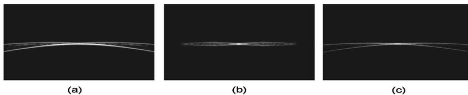
FIG. 5. B-mode images of a point target placed on the  $z$  axis at 60 mm. The full transmit aperture was applied with a fixed, 40-mm focal length but only the center transducer element was used to receive echoes (a). Applying a 2D matched filter to the rf echo signal in (a) results in the image of (b). (c) is the image constructed also from center receive element but where the transmit focus was moved to 60 mm (DRF-focus result).
