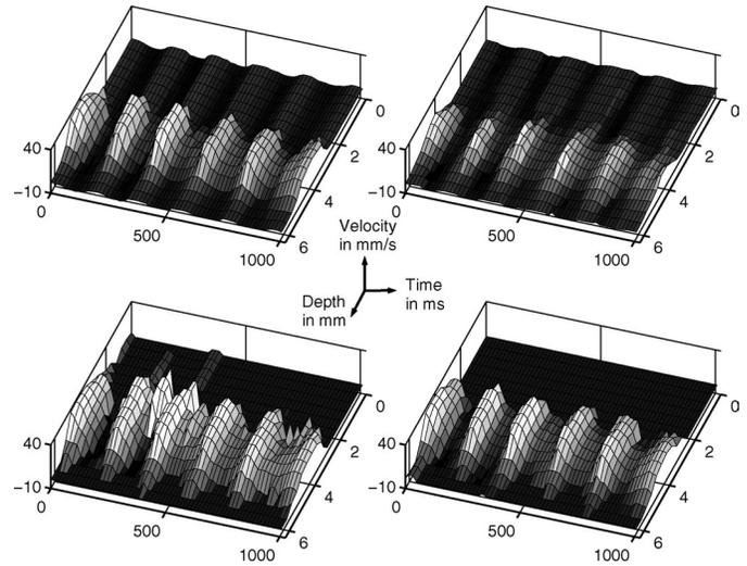
Fig. 6. Different filters were applied to suppress tissue motion: zero-initialized second-order IIR (top left), step-initialized second-order IIR (top right), first-order regression (bottom left), and first-order eigenfilter (bottom right).
