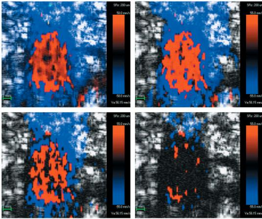
Fig. 13. 2-D CF images where the flow and clutter Doppler shifts are equal in magnitude and opposite in sign. Unfiltered (upper left) and second-order projection-initialized IIR filter with 3 increasing cut-off frequencies (highest value lower right) and  $N = 8$ . The length of the green bars in the lower left corners represents 1 mm.
