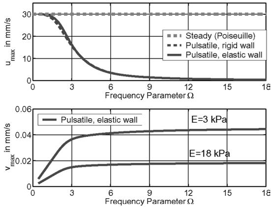
Fig. 5. Computed maximum axial fluid and radial wall velocities in an elastic tube (radius  $a = 3$  mm,  $h/a = 0.1$ ,  $\nu = 0.5$ ) for a frequency-independent pressure gradient  $k_s = -13.3$  N/(m<sup>2</sup>·m) as a function of the frequency parameter  $\Omega$  and elastic modulus  $E$ . See the Appendix.
