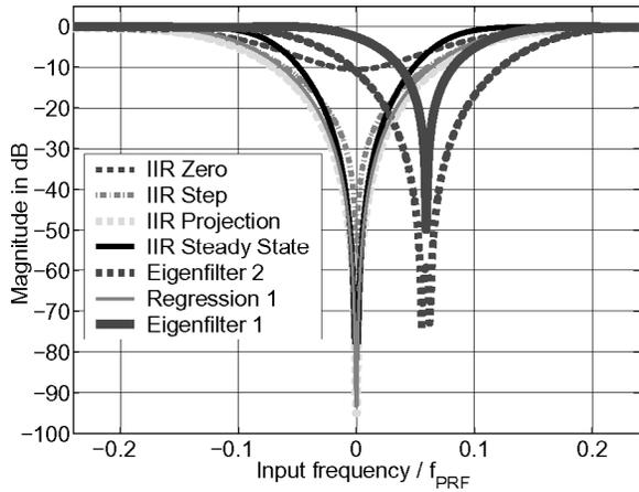
Fig. 7. Filter frequency responses in the range of  $-0.25f_{\text{PRF}}$  to  $+0.25f_{\text{PRF}}$  for  $N = 8$ . The second-order IIR Chebyshev filters are highpass with a cut-off frequency of  $0.0755f_{\text{PRF}}$  Hz. The eigenfilter was designed to suppress clutter centered at  $+0.0566f_{\text{PRF}}$ . Increasing the order of the eigenfilter also increases attenuation but widens the stopband.
