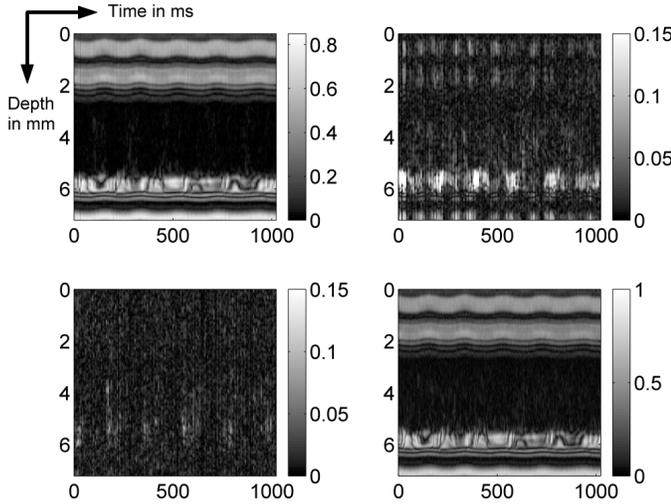
Fig. 9. Separate eigencomponents are shown in an M-mode format when the clutter is from moving scatterers. In the top row are the brightness eigenimages related to the first (left) and second (right) eigencomponent. The bottom row shows the 3rd eigencomponent (left) followed by the combination of all eight (right). Note the different brightness scalings. Clutter is contained in the first two eigenimages.
