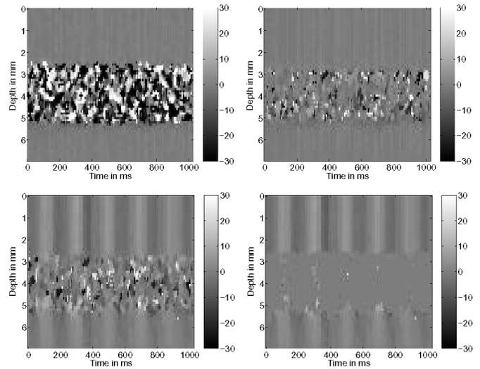
Fig. 11. Displacement images of M-mode data. Top row are for stationary clutter and bottom row for moving clutter. Top left is unfiltered, while the remaining images are filtered using a first-order eigenfilter. These images demonstrate that tissue motion can be estimated independent of flow. The colorbar is scaled in microns.
