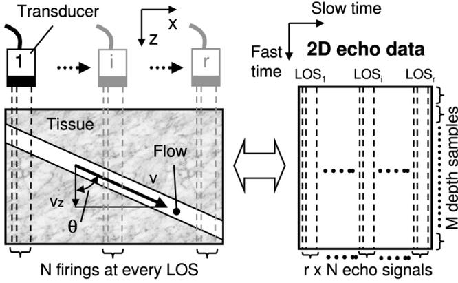
Fig. 1. Scan-mode acquisition for CF imaging (left) and matrix representation of data (right). Matrix dimensions are  $M \times rN$ . The situation for M-mode is similar except there is no transducer motion along the  $x$ -axis ( $r = 1$ ), and only a single LOS is investigated as a function of time.
