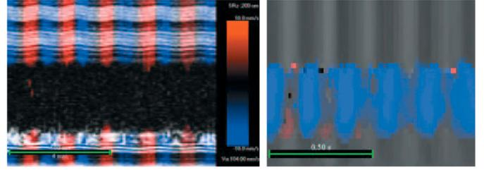
Fig. 15. Left: CF image where only the first eigencomponents are used to estimate velocity from the 2-D autocorrelator. Right: Corresponding displacement-flow image where displacement is computed from the first eigencomponent only. Flow is derived from all but the first eigencomponent. The length of the green bars in the lower left corners represents 500 ms (horizontally) and 4 mm (vertically).
