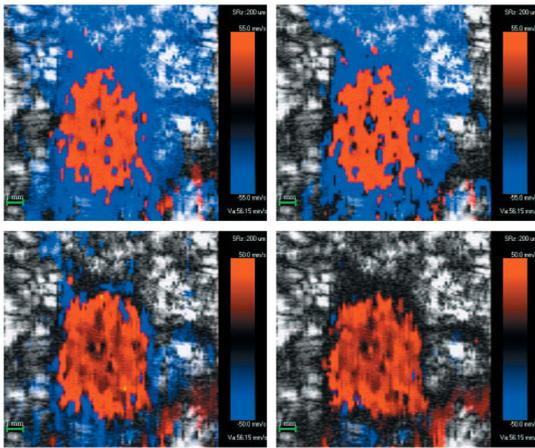
Fig. 14. 2-D CF images for first-order (upper left) and second-order (upper right) polynomial regression filters. In the bottom row are the results for a first-order (lower left) and second-order (lower right) eigenfilter with  $N = 8$ . The length of the green bars in the lower left corners represents 1 mm.
