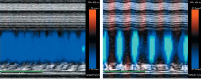
Fig. 12. Left: Color M-mode image shows steady flow in the 3-mm-diameter flow channel away from the transducer with the pulse channel off. Right: Color M-mode image of the same channel temporally modulated by the adjacent pulsed-pressure channel. The color scales of both images are the same. Cyan regions indicate velocities away from the transducer that are out of range. Clutter appears as color outside the channel.
