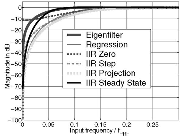
Fig. 3. Frequency responses of HP filters ( $N = 8$ ). The maximum (aliasing) frequency is  $0.5 f_{\text{PRF}}$  (not shown). Second-order IIR Chebyshev filters were designed with a cut-off frequency of  $0.0566 f_{\text{PRF}}$  Hz to match the  $-3$  dB point of the eigenfilter designed for stationary clutter signals (zero Doppler shift).
