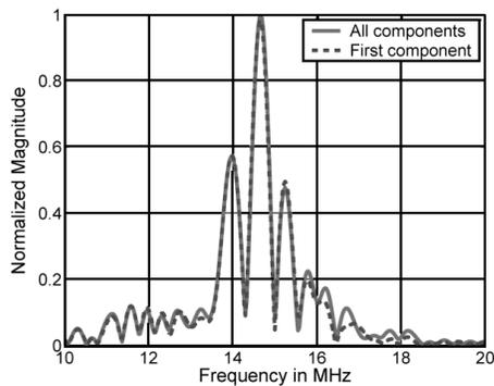
Fig. 10. Fast-time spectra of the clutter component computed from a single pulse packet in the upper part of Fig. 9: all 8 eigencomponents (no filtering) and the first eigencomponent only.
