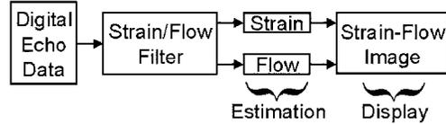
Fig. 2. Block diagram of combined strain-flow imaging.
