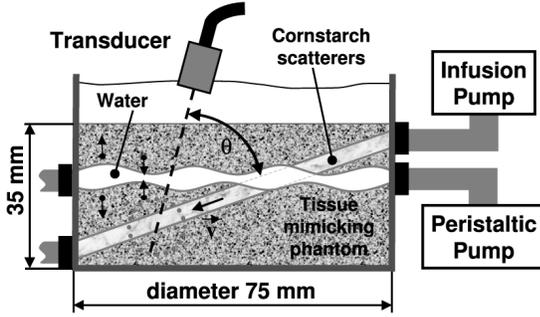
Fig. 4. Phantom experiment for generating clutter. Echo data were acquired in M-mode in the vicinity of the circled region.
