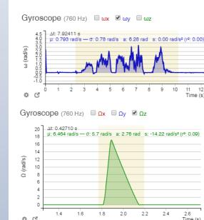
Example calibration activity data with analysis tools. Students find angular displacement using the area under the curve of the highlighted area ("a").
