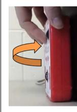
Students are guided to rotate the IOLab to check the calibration of their gyroscope sensor.
