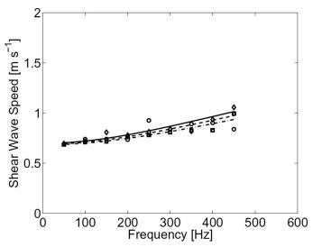
Fig. 7. Measurements of shear wave dispersion in one 4% gelatin sample for actuator voltages set to 5, 10, and 15 V. Lines are best-fit dispersion models used to estimate the complex modulus. Equivalence of the three responses demonstrates the linear mechanical response of the gelatin gel.
