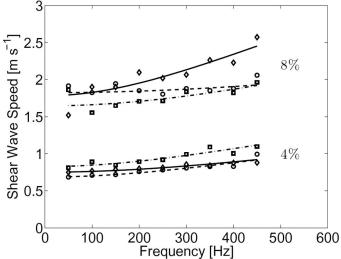
Fig. 6. Measurements of shear wave dispersion in six samples, three each with 4% and 8% gelatin concentration. Lines are best-fit dispersion models used to estimate the complex moduli listed in Table I. For both concentrations, measurements from sample 1 are indicated by a circle, sample 2 by a diamond, and sample 3 by a square.
