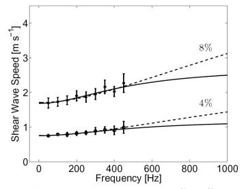
Fig. 8. Average shear-wave dispersion measured for 4% and 8% gelatin concentrations and best-fit model curves. The dashed lines are for the Kelvin-Voigt model and solid lines are for the Zener model. Error bars indicate one standard error based on measurements from three samples each.
