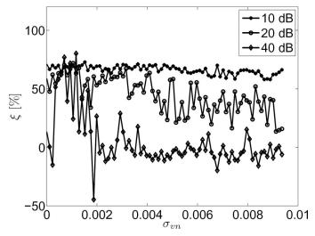
Fig. 4. Percent improvement  $\xi$  is plotted as a function of normalized Doppler spectrum width  $\sigma_{vn}$  for 10, 20, and 40 dB echo SNR ratio. Results are from simulated echo data.
