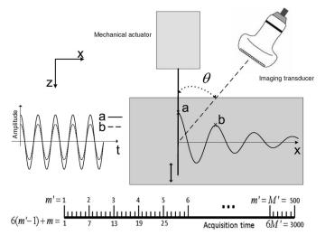
Fig. 1. Diagram of the experiment to measure viscoelastic properties of gel samples. Mechanical actuator is driving a stainless steel needle. Momentum of the needle displacement is transferred to the medium as cylindrical shear waves. A linear array Doppler probe tracks the induced transverse motion of scatterers as shear waves propagate. At the bottom is a timing diagram for the (up to) 3000 Doppler pulses transmitted at each position along x.
