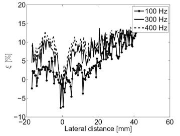
Fig. 5. Percent improvement  $\xi$  is plotted as a function of lateral distance from the source for 100, 300, and 400 Hz shear wave frequencies. Results are measured from gelatin gels.
