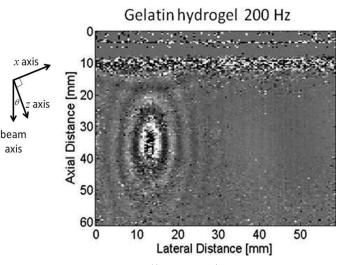
Fig. 2. Particle velocity image  $\hat{v}(x\cos\theta, z\cos\theta)$  in gelatin from one RF frame. Shear waves are generated by a needle moving near the elliptical center. The x, z axes (Fig. 1) are rotated  $\theta = 30^{\circ}$  counterclockwise about the needle.
